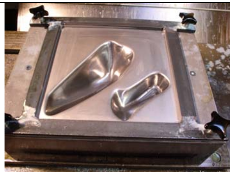
Upper muffler part made with SPIF
