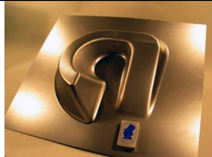
Upper muffler part made with SPIF
